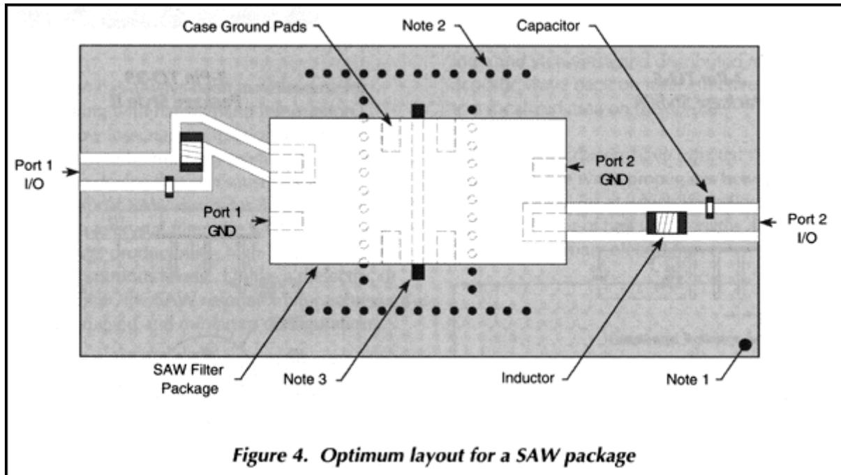
**Figure 4. Optimum layout for a SAW package**
