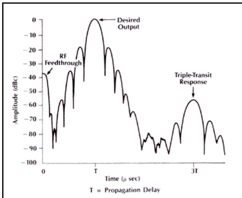
Figure 1. Impulse response of a typical SAW filter
